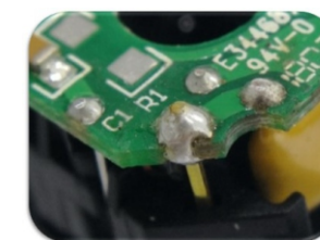
异型焊盘焊接 Deformed Pad Soldering
