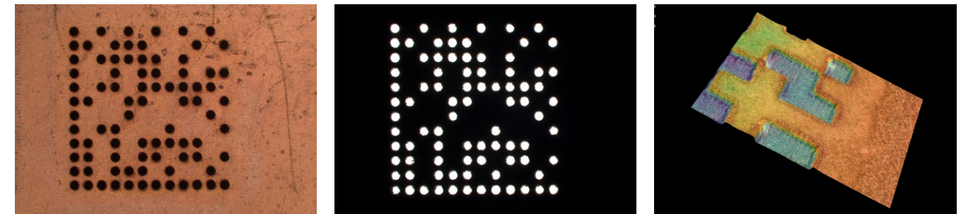
通孔0.15孔径，DM码 Through hole 0.15 the aperture, DM code
