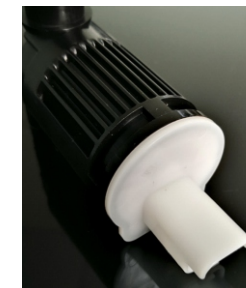
915nm激光 水泵壳体焊接 915nm Laser Water pump shell welding
